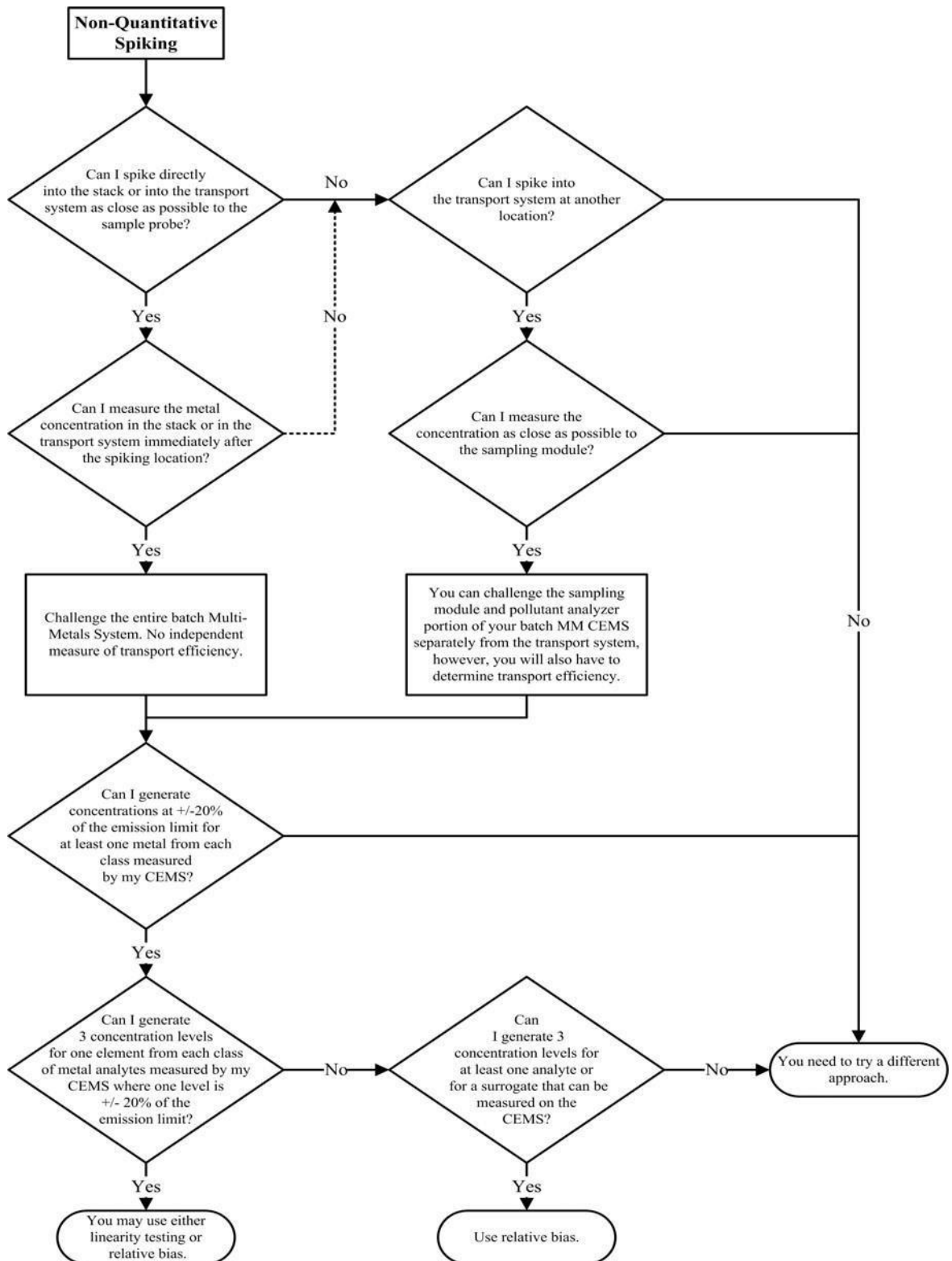
Figure 3: Flow chart for using non-quantitative spiking during the accuracy tests.
